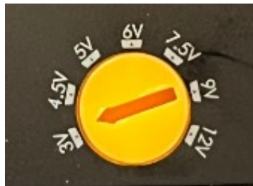
Voltage selector switch
