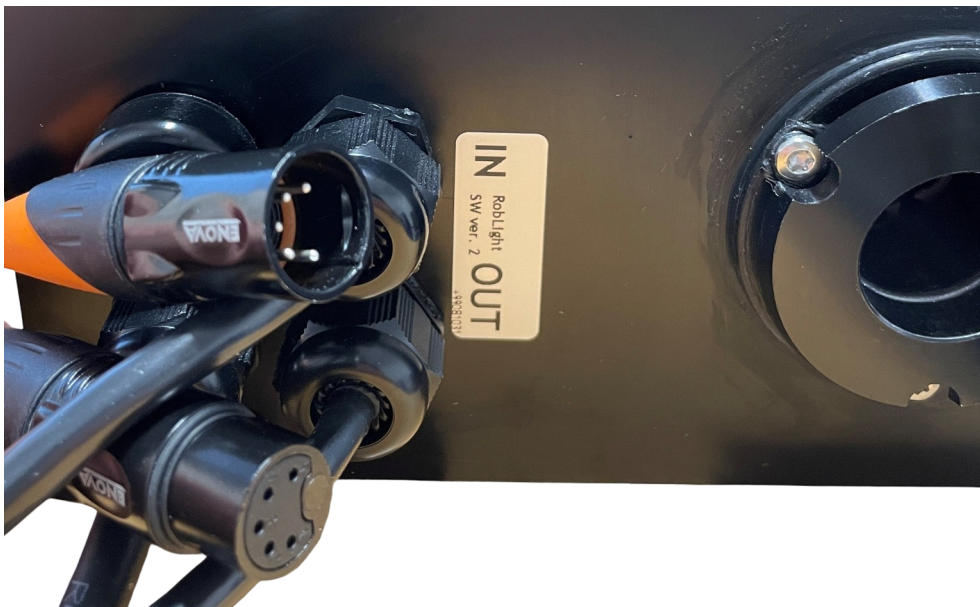
Figure 1 - DMX input (male) and output (female) connectors.
